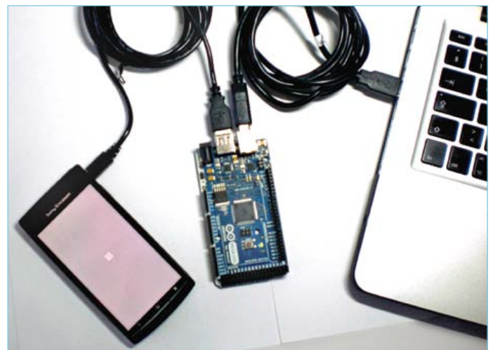
Figure 2. Arduino Mega ADK connected to a PC and to a phone.
