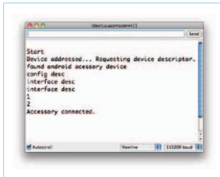
Figure 3. Screenshot from the Serial Port Monitor when linking an Android device to your Arduino Mega ADK.
